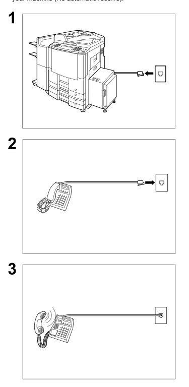
Unplug the Telephone Line Cable from the telephone jack that was supplied by the telephone company.
